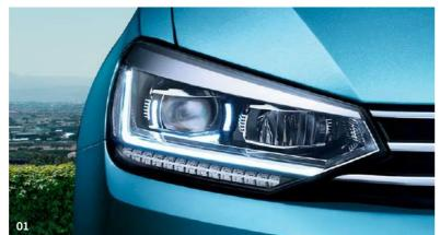
01 LED premium headlights provide optimum road illumination by producing a light that is brighter than conventional halogen headlights. Also featured with this option is projection technology, LED daytime running lights and rear tail lights, and dynamic cornering lighting. Optional on SE models and above. Model shown features optional metallic paint.
